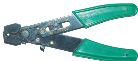
Stripping tool SCT001, cuts and strips 0.5-6 mm 2
